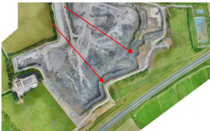
Figure 19 Areas where bund height should be increased
